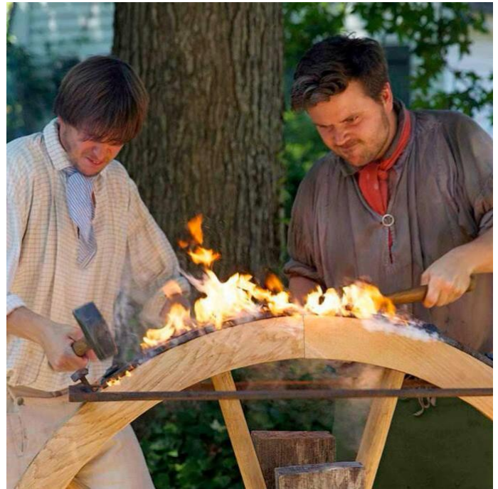
Master wheelwright Phill Gregson and Andre De Lisle nailing strakes to traditional wooden canon wheels. From worldwidewheelwright.com
