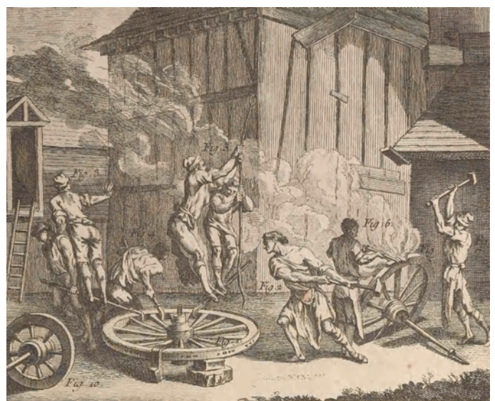
Figure 4. Wheelwrights applying the tyre . From Diderot's Encyclopédie (1751-66)
